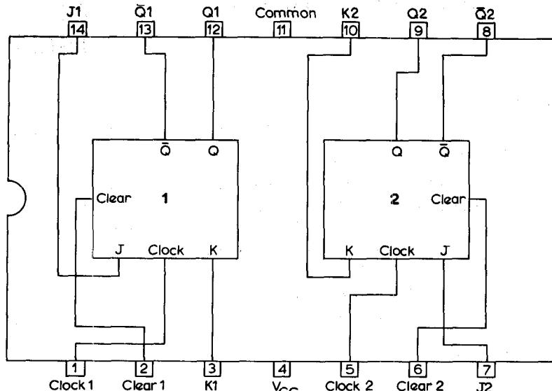
'Low' input to clear sets Q to logical '0' regardless of clock state
